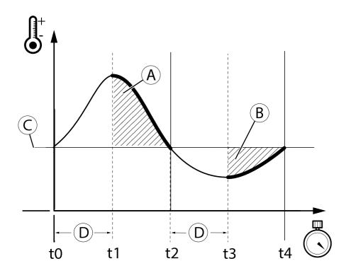
4. If detection type Above (A) or Below (B) is selected: Enter a Delay Time (D) in seconds.
